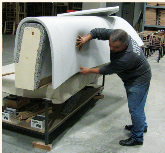
A craftsman works to wrap sofa foam at Stella's Istanbul manufacturing facility.
