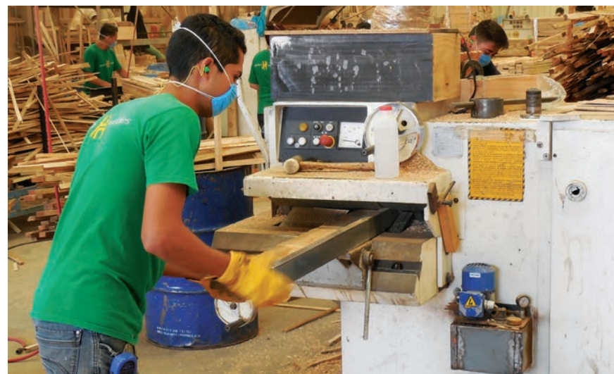
A worker guides a board through a planer in the machine area.
