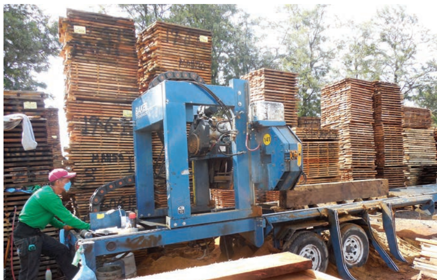
A worker cuts boards in the lumberyard outside the plant in Zapopan.
