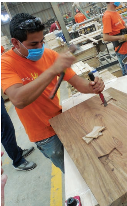
A worker uses a hand chisel to carve a space for butterfly joints on a dining table top.
