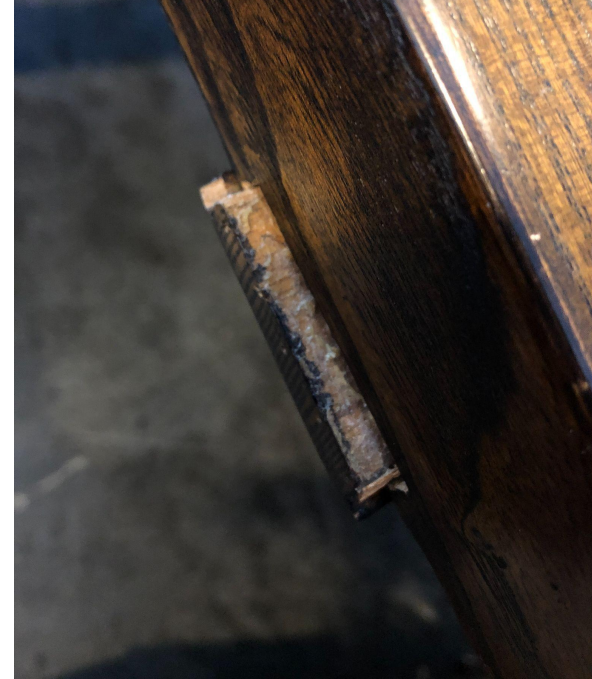
An early table with a wood beam jutting from the side after warping. Maria would spend the next ten years reengineering joinery techniques to completely eliminate such issues
